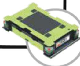
From the store, kits once prepared are **transported as unit load** by mobile robots to respective sub-assembly stations
